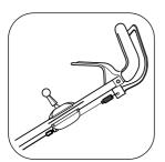
Unscrew the locknuts and screw the adjuster in or out as necessary. Tighten the locknuts when correctly.
